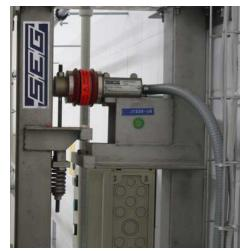
The weighing unit consists of two vertical members interconnected by two accurately matched, parallel flat springs. These are rigid in all directions except the vertical one. One of the members is fastened to a rigid, vertical surface and the other to the load carrier. The two uprights are also connected to the load cell via a bar arrangement so that the cell takes up the vertical force only.
