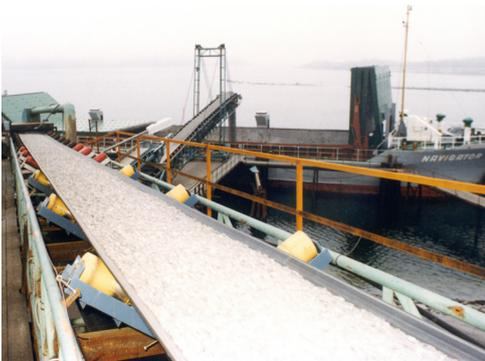
The weighing units can be installed in any ordinary conveyor with minimal disruption of operation. The number of weighing units installed is based on the accuracy requirements.
